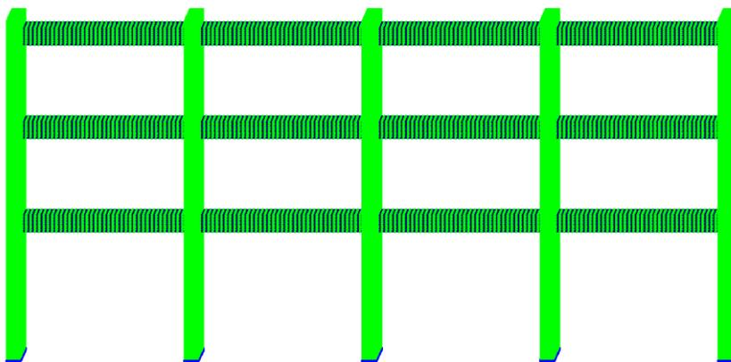
**Fig. 4.** General view of the finite element model of reinforced concrete frame in LIRA-CAD software
