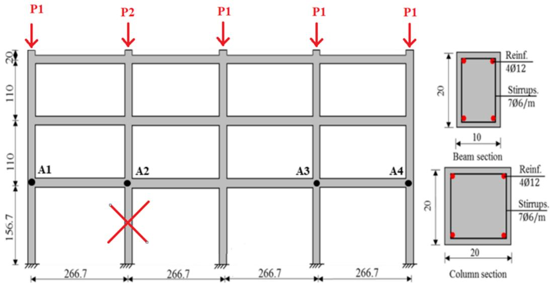
**Fig. 3.** Dimensions and reinforcement scheme of reinforced concrete frame sections (cm)
