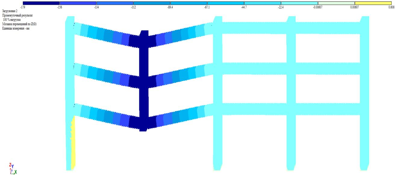
**Fig. 5.** Deformed state of the reinforced concrete frame at the calculation iteration preceding the structural collapse
