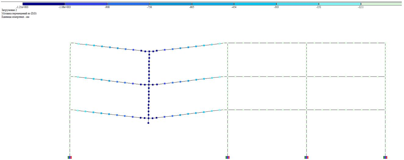
**Fig. 8.** Deformed state of the structural finite element model of the reinforced concrete frame
