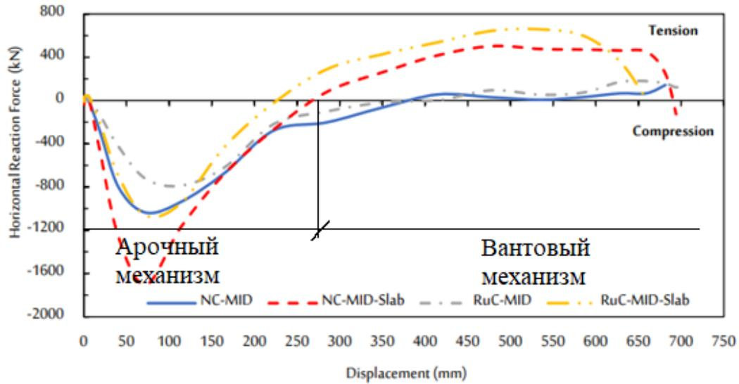
**Fig. 1.** Relationship between axial force and deflection of the beam [5]
