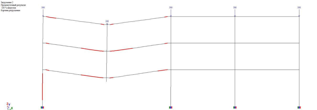
**Fig. 9.** Fracture pattern of the bar finite element model of the frame
