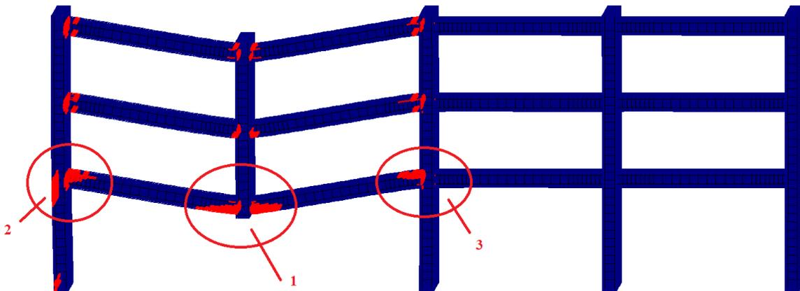
**Fig. 6.** Fracture patterns of reinforced concrete frame model
