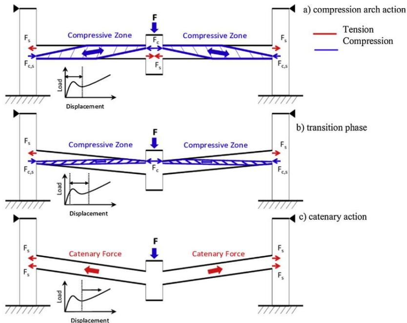
**Fig. 2.** Arch and catenary resistance mechanism [6]
