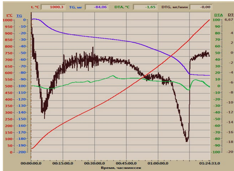
Fig. 10. DTA of hydration products “aspiration cement dust – volcanic tuff – \text{Na}_2\text{SiO}_3 – sodium fluorosilicate.
