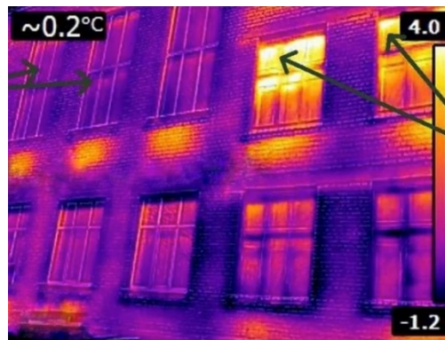
Fig. 1. Heat loss through translucent structures in a residential apartment building.
