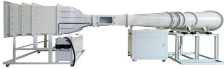
Fig. 10. Low-speed direct-current aerodynamic tunnel.
