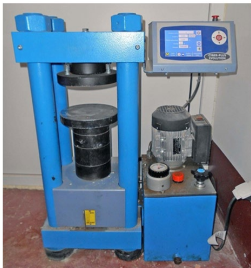
Fig. 2. Press for testing concrete strength by destructive method.
