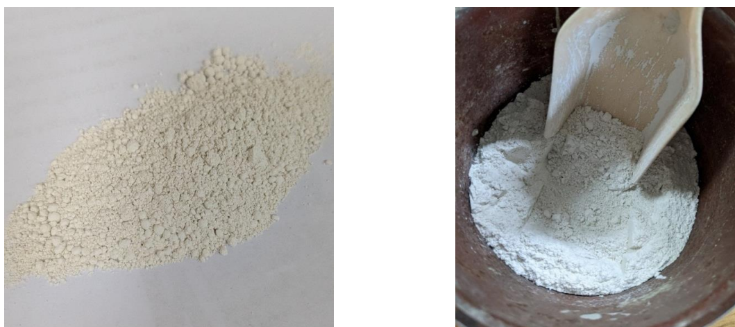
Fig. 8. Dihydrate technogenic gypsum after grinding.
