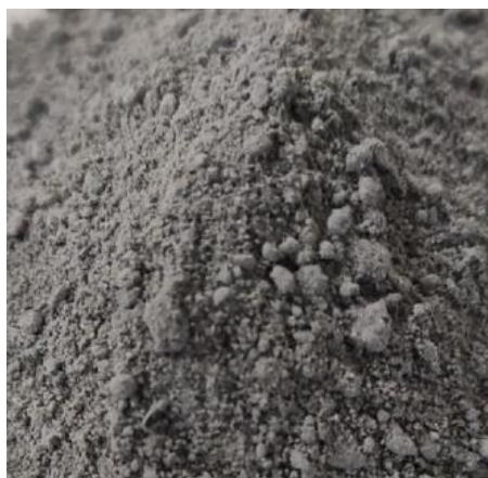
Fig. 11. Appearance of man-made basalt powder. Fig. 12. Microstructure of man-made basalt powder.
