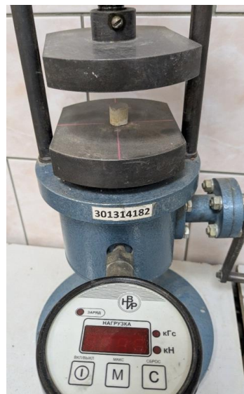
Fig. 3. Laboratory hydraulic press with measuring scale.
