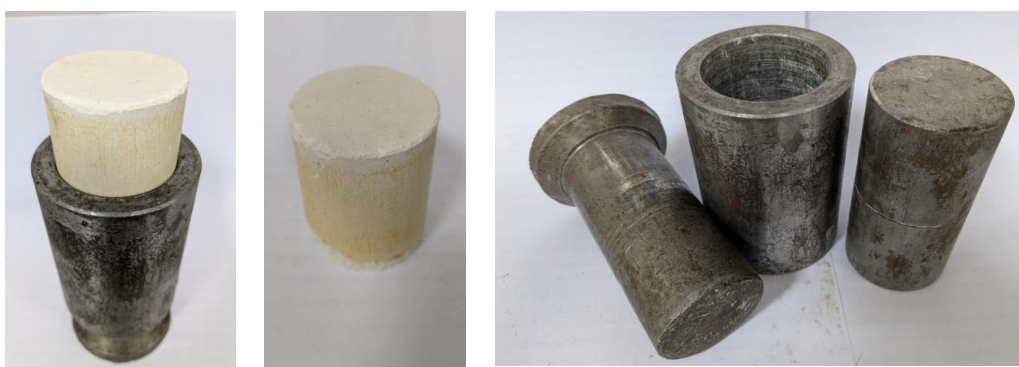
Fig. 1. Sample after pressing and mold for pressing.
