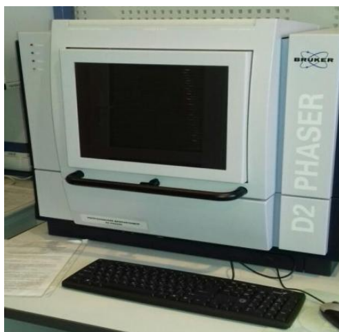
Fig. 3. BRUKERD2 PHASER X-ray diffractometer.
