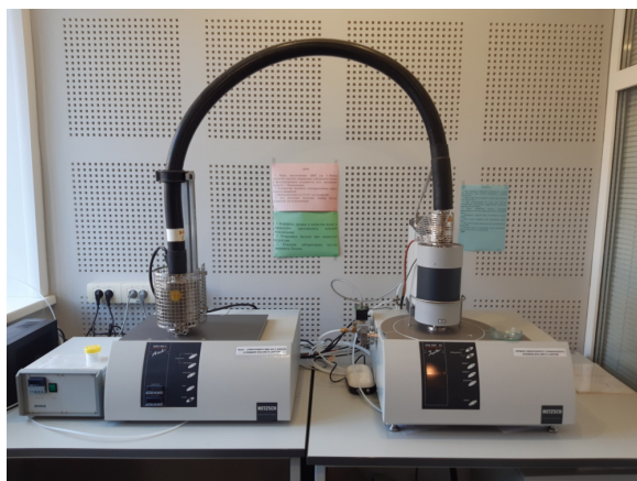
Fig. 6. STA 449 F1 Jupiter® synchronous thermal analysis (TG-DSC) instrument with QMS 403 CF Aeolos mass spectrometer.
