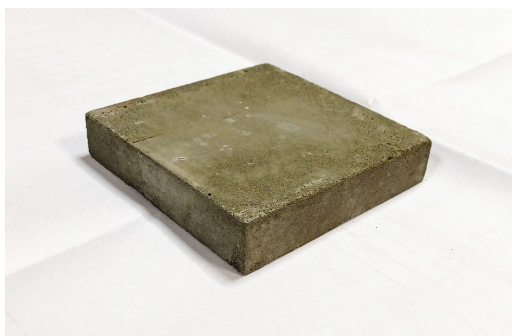
Fig. 4. General view of the foam concrete sample for determining the thermal conductivity coefficient.
