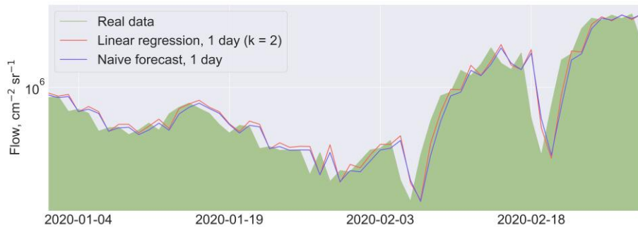
Figure 17. Forecast of >2 MeV daily integral electron fluxes for 1 day
