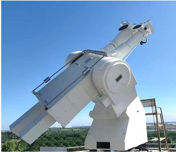
Figure 1. General view of the SFMM telescope at Gan Yu Solar Station of the Purple Mountain Observatory, Jiangsu Province. At the right bottom corner is a strip with sea
