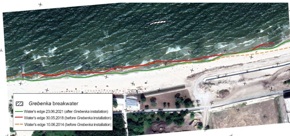
Fig. 6. Interannual dynamics of the water's edge near the breakwater before and after its installation (2014 – GoogleEarth source, 2018 – satellite image ResursP, 2021 – GPS tracing)
