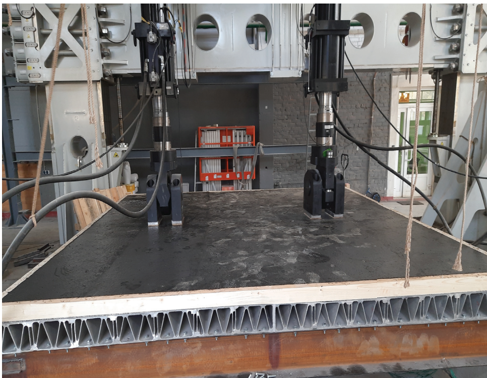
Fig. 10. Paired orthotropic slabs with asphalt concrete coating on the test bench for static and fatigue tests
