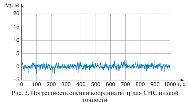
Fig. 3. Coordinate \eta estimation error for low accuracy satellite navigation systems
