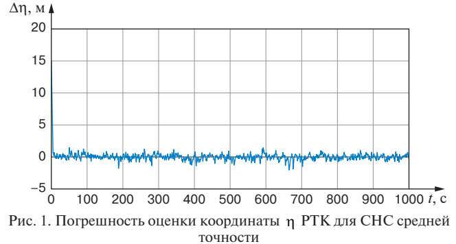
Fig. 1. Coordinate \eta estimation error of robotic systems for medium accuracy satellite navigation systems
