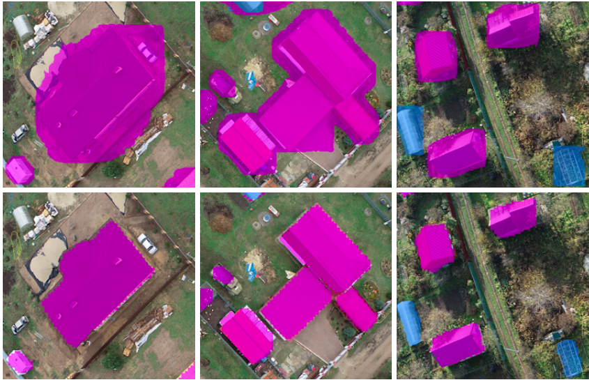
FIGURE 9. The results of GAN enhancement are shown under the Mask R-CNN predicted real estate object masks
