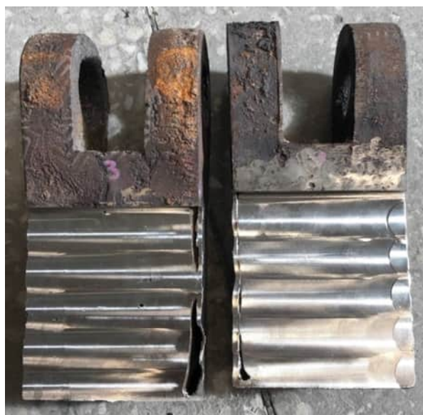
Fig. 5. Extended through-thickness defects on the beater, numbered 1, 3 (see Fig. 3)
