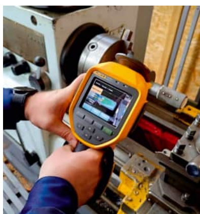
Fig. 7. Verification of temperature readings obtained from thermocouples using the FLUKE Ti400 thermal imager:
