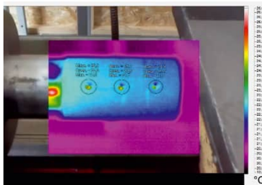
Fig. 7. Verification of temperature readings obtained from thermocouples using the FLUKE Ti400 thermal imager:
