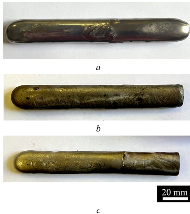
Fig. 1. Photographs of ingots 1 (a), 2 (b), and 3 (c) of TiNiHf SMA after vacuum arc melting with 8-fold remelting
