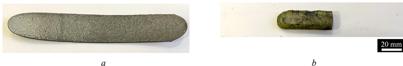
Fig. 3. Photographs of the obtained sheet from ingot 2-1 ( TiNiHf alloy) with a thickness of 2.2 mm (a) and ingot 3-1 after fracture (b)
