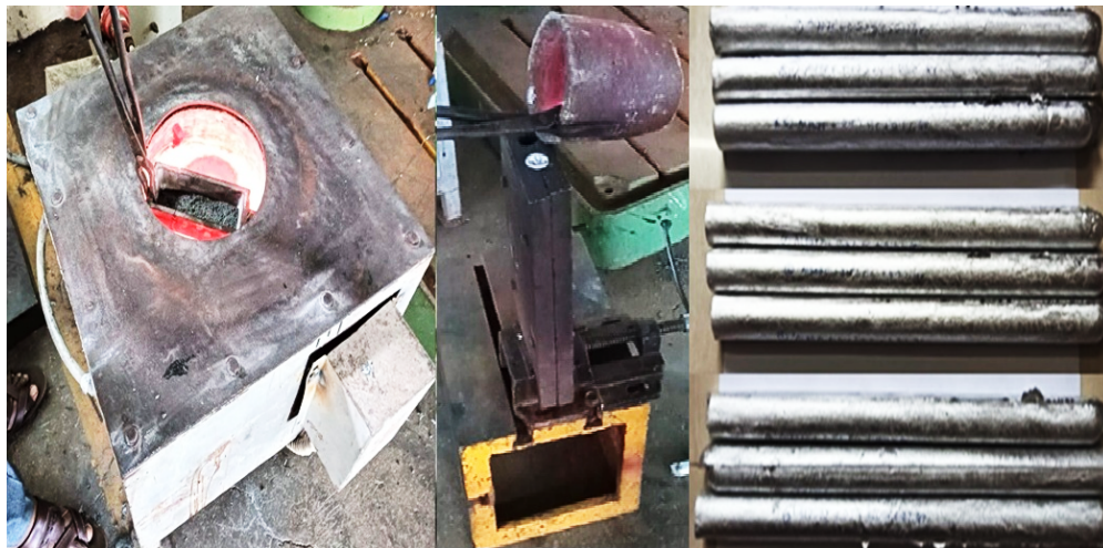
Fig. 1. Preparation of Al7075 specimens with varying reinforcements by stir casting
