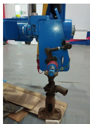
Figure 8. Method of adjusting the angle of installation of the strain gauge pin in the "zero" position using a pull bar of variable length Source: made by A.A. Karsakov
