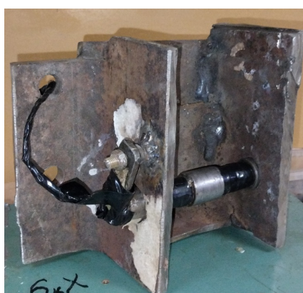
Figure 7. Installation of the strain gauge pin in the found position and locking it against rotation relative to the longitudinal axis Source: made by A.A. Karsakov
