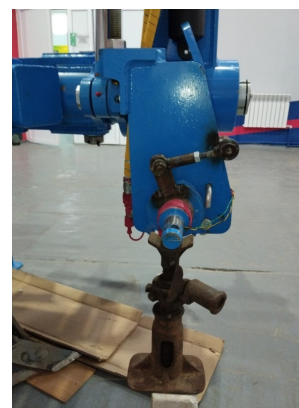
Figure 8. Method of adjusting the angle of installation of the strain gauge pin in the "zero" position using a pull bar of variable length
