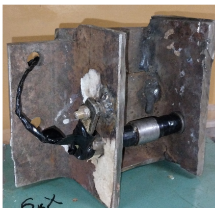
Figure 7. Installation of the strain gauge pin in the found position and locking it against rotation relative to the longitudinal axis
