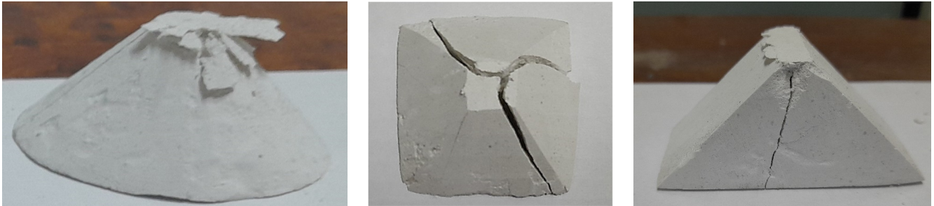
Figure 4. Test results of the specimens of the first group, brought to fracture Source: made by A.V. Masalov
