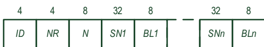
Fig. 3. NACK Packet; ID) Packet Identifier 4 Bits; NR) Node Identifier 4 Bits; N) Number of NACK Repeats 8 Bits; SN) Sequence Number of the First Lost Packet in Succession 32 Bits; BL) Burst Length 8 Bits
