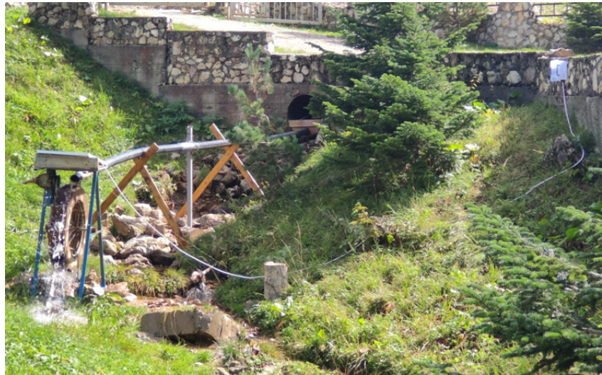
Figure 3. Autonomous installation for collecting microhydropower parameters.
