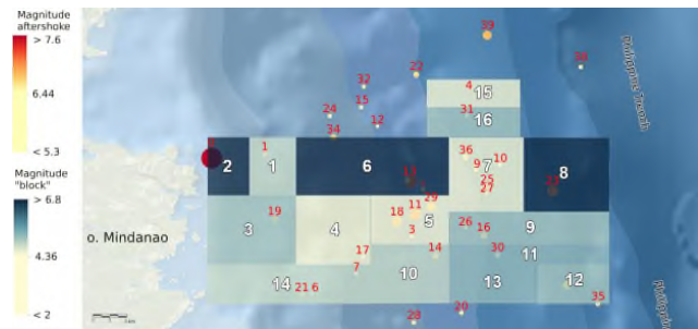
Figure 5. Visualization of the constructed earthquake source for the first scenario, where the big red point is corresponds to the epicenter of the earthquake; orange and yellow circles correspond to aftershocks of the earthquake.
