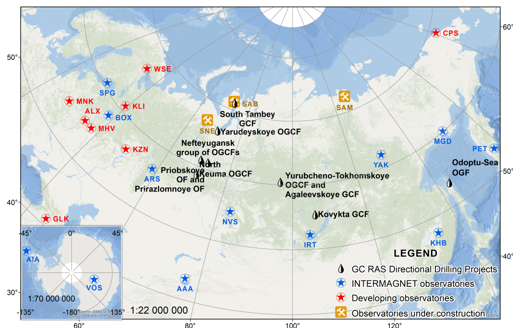
Figure 4. Map of oil and gas fields where GC RAS provides geomagnetic support technology for directional drilling, and magnetic observatories in Russia and neighboring countries, which transmit data to Analytical Geomagnetic Data Center at GC RAS.
