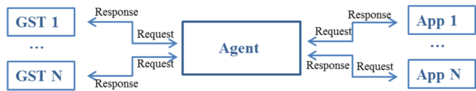
Figure 2. Scheme of interaction of GST instances and external applications.
