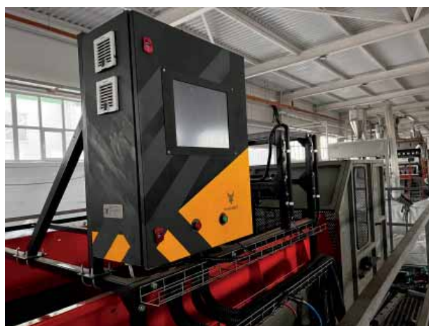
Fig. 2. Appearance of the WINGSBEE separator installed on the technological line of the waste sorting complex.
