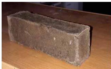
Fig. 6. Saponite-basalt structural and thermal insulation composite
