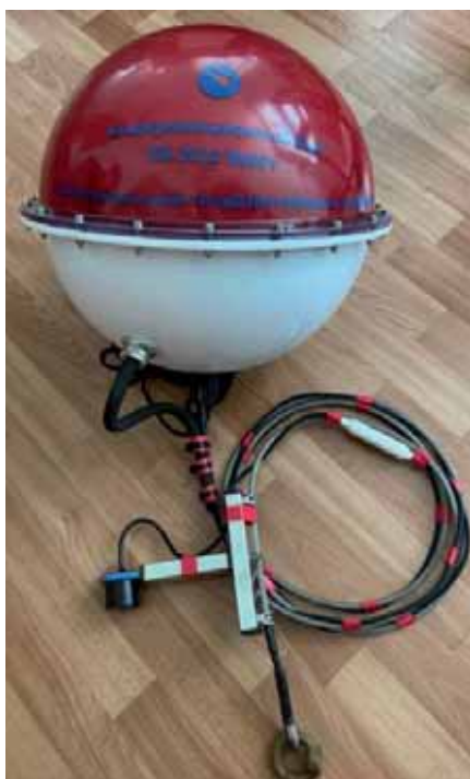
Fig. 5. Marine communication buoy with combined underwater and surface communication facilities.
