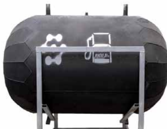
Fig. 5. Biofuel Production Reactor, diameter 950 mm, length 1500 mm
