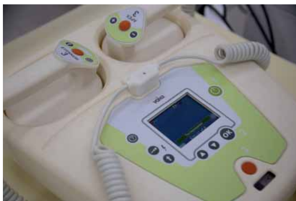
Fig. 3. Automatic external defibrillator with built-in human condition diagnostic system.
