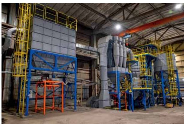
Fig. 3. Complex for grinding metallurgical waste to produce mineral powders MP-2.
