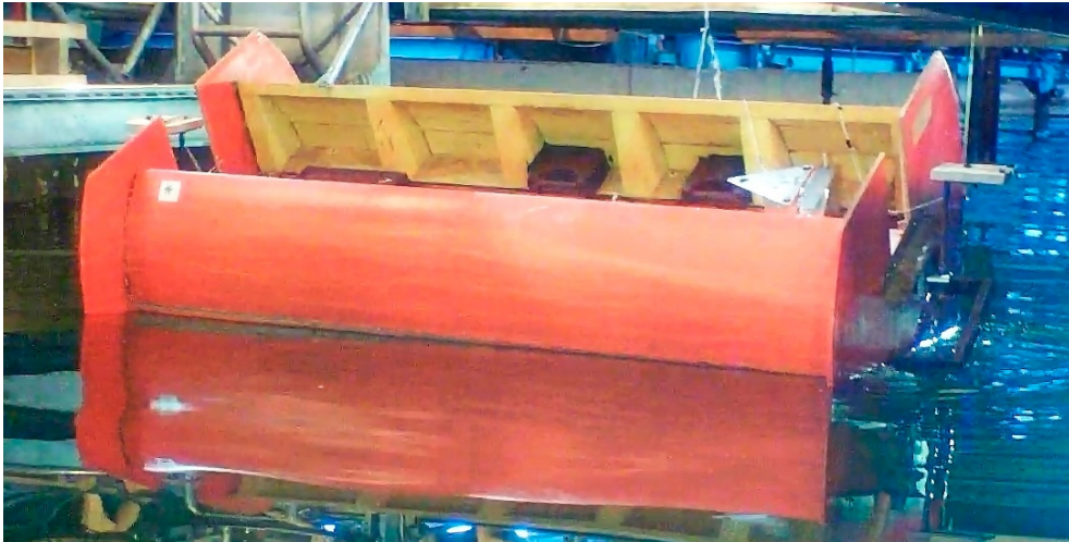
Fig. 11. Model during wave tests in the experimental wave basin
