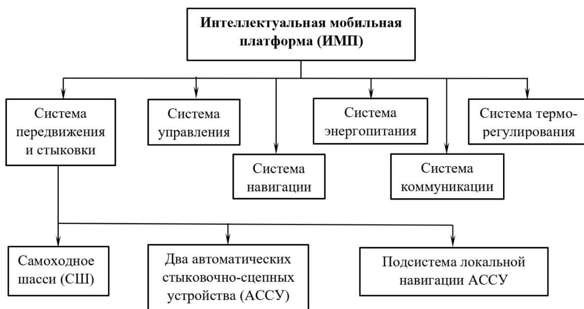
Figure 6. Structural diagram of the intelligent mobile platform.
