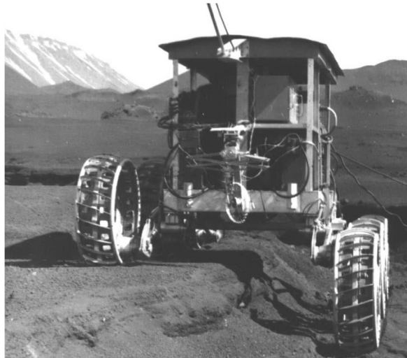
Fig. 8. Fragment of tests of the experimental sample of self-propelled automatic landing gear at adjusting the relative position of wheels and body vertically in the area of recent eruptions of the Tolbachik volcano in Kamchatka.
