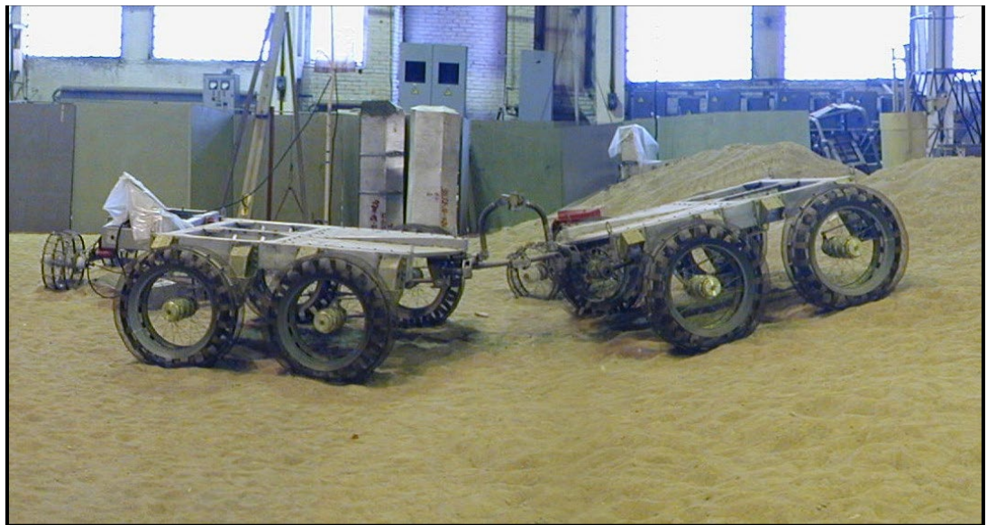
Fig. 1. Running mockup of the two-section self-propelled landing gear of the manned lunar rover (from the author's archive).
