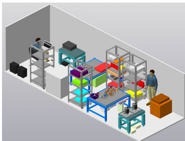
Fig. 1. Designed arrangement of OFS components in a van. The van is divided into three compartments, viz. operator compartment, OFS physical part compartment, and frequency measurement compartment. The operator compartment contains a personal computer with a control system and uninterruptible power supplies. The OFS physical part compartment houses the optical spectroscope, radiation distribution scheme, and auxiliary equipment. The last compartment contains highly stable laser systems and femtosecond optical frequency synthesizer.
