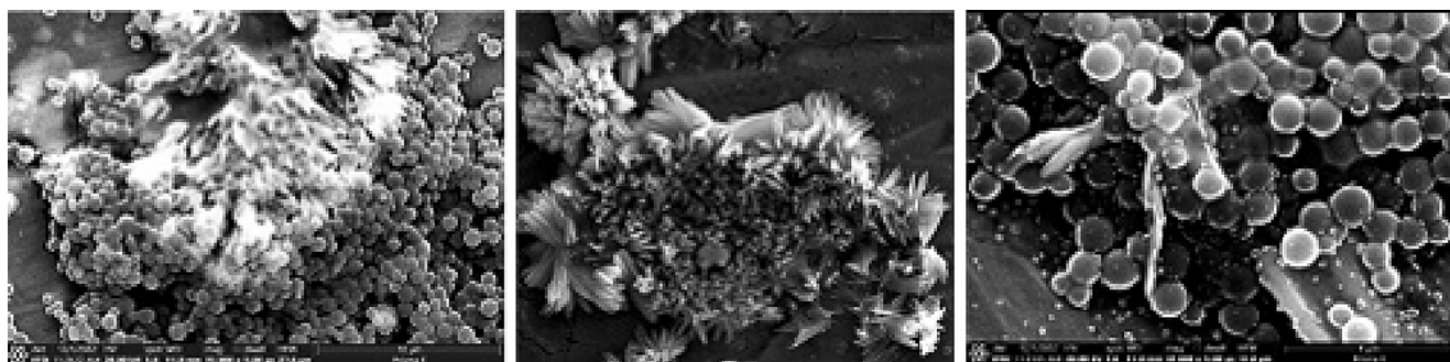
Fig. 7. Electron microscopic photographs of polystyrene latex synthesized in the presence of 6% CA in styrene.
