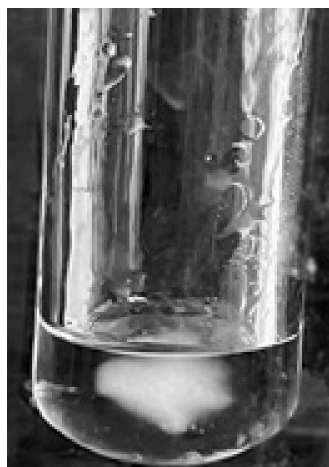
Fig. 5. Appearance of CA crystals in styrene block copolymer when the temperature is lowered to 5°C.
