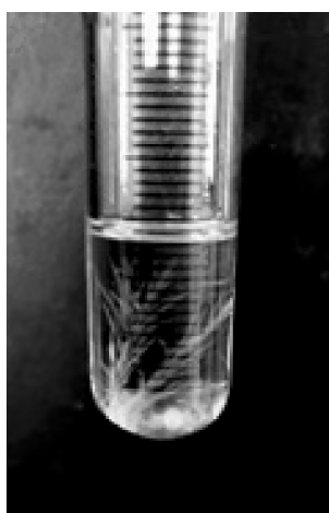
Fig. 6. Crystallization of CA in styrene when the solution temperature is lowered to 5°C. The concentration of CA in styrene is 6%.
